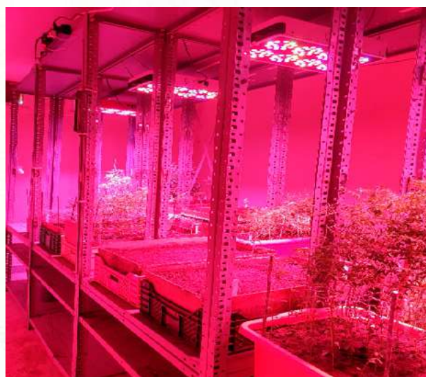
Figure 1: Speed breeding growth chamber
